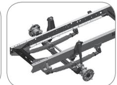
Front Parabolic Suspension and Rear Semi-elliptical Suspension
